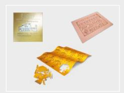
There is not enough room to show all the applications which can be professionally processed with the LPKF ProtoLaser U4. A small sample, from left: processing of metal layers on  $Al_2O_3$  (with 40  $\mu$ m drill holes); flexible and rigid circuit board processing (structuring, cutting, drilling).
